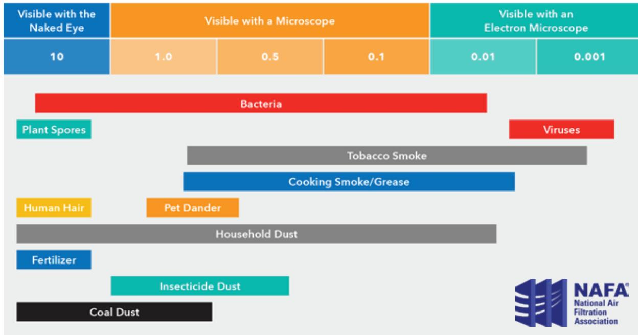
evenly dispersed through the supply vents into the occupied space. Mold and bacteria predominantly fall into the 0.3 - 3.0 micron range, the particulate size range most important to containment. This is the size likely to be liberated and entrained in the air flow whenever the building envelope, plumbing, electrical, mechanical systems, or finishes are disturbed. Humans don't begin to see particles with our naked eyes until the 10 micron size and larger.
