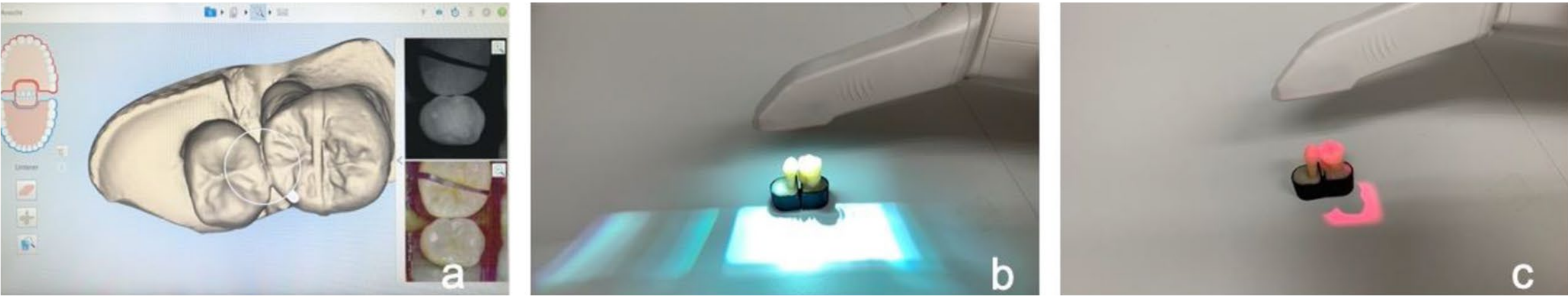
Fig. 1 – The application of the three-dimensional near-infrared reflection scanner is visualized by a monitor with the appropriate software (a). The tooth is illuminated either with a white LED (b) or a red laser (c)
